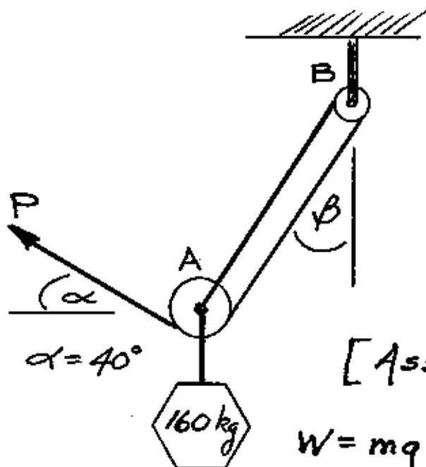
A 160-kg load is supported by a rope and pulley system.
