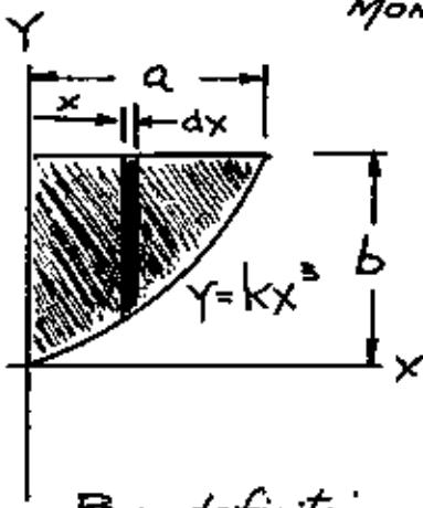
MOM. of INERTIA with respect to Y-AXIS
