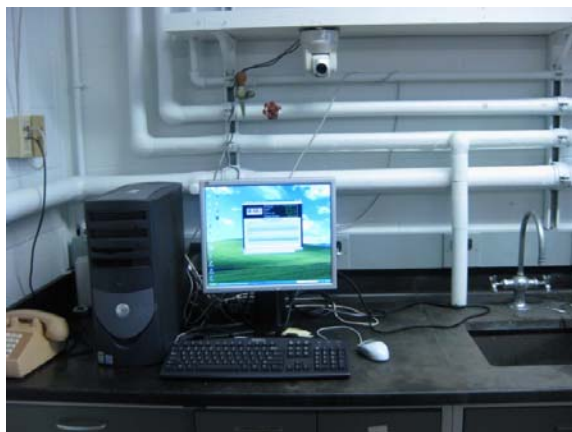
Fig. 1.1. PPMS laboratory analysis computer with temperature and humidity logging sensor. Above the monitor is a network camera (sound, pan by 350°, tilt by 120° and 22x zoom) which enables one to remotely monitor conditions in the room. In concert with the ability to remotely login to the control computer, the camera enables one to conduct experiment at a location remote from the laboratory.
