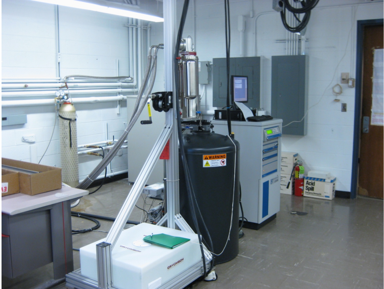
Fig. 1.3. View of the helium recovery closed cycle system (chrome cylinder) attached to the aluminum rack, the large capacity dewar (black cylinder) for the PPMS system and control cabinet and control system. In the far corner, you can see the reservoir for the split chilled water system (heat exhaust part on roof).
