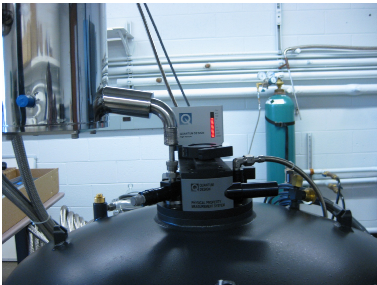
Fig. 1.4. Close-up view of the helium vapor extraction probe inserted into the PPMS liquid helium reservoir. Vapor is condensed in an internal cold head (in chrome cylinder) and reinjected into the helium reservoir in standard operation mode. In fill-mode, room temperature helium gas from a standard tank (background) can be converted into liquid helium to top-off the reservoir as a result of loss of liquid helium from rapid boil-off when the magnet is continually ramped.
