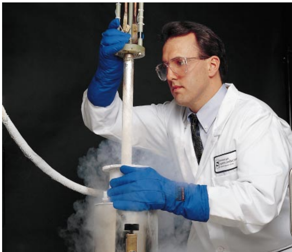
ANOTHER DAY, ANOTHER DOLLAR: a technician from American Superconductor removes a BSCCO cable from a dewar of liquid nitrogen for testing. In most envisioned applications, cryocoolers rather than liquid nitrogen will be used.
