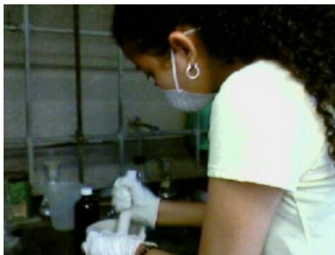
**Fig. 4.** Sample components mixed and then ground to a fine grey powder.
