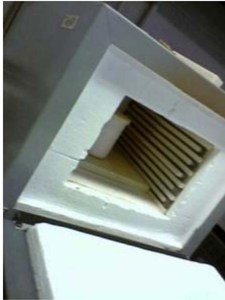
**Fig. 5.** Sample placed in Alumina crucible with lid for calcination (firing at high temperature  $\sim 950^{\circ}\text{C}$ ) in high temperature furnace.
