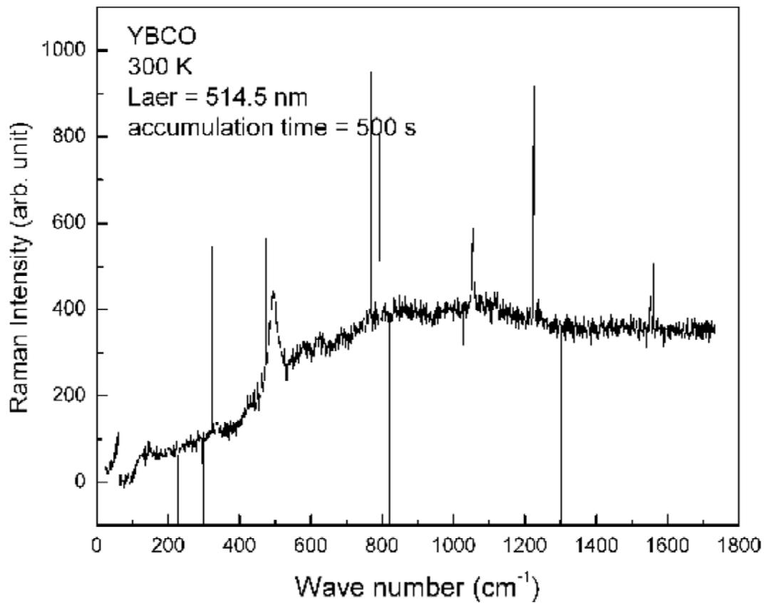
**Fig. 12.** Raw Raman data with sharp singlepoint spikes from cosmic ray hits. Measurements conducted in Prof. T. Zhou's lab.
