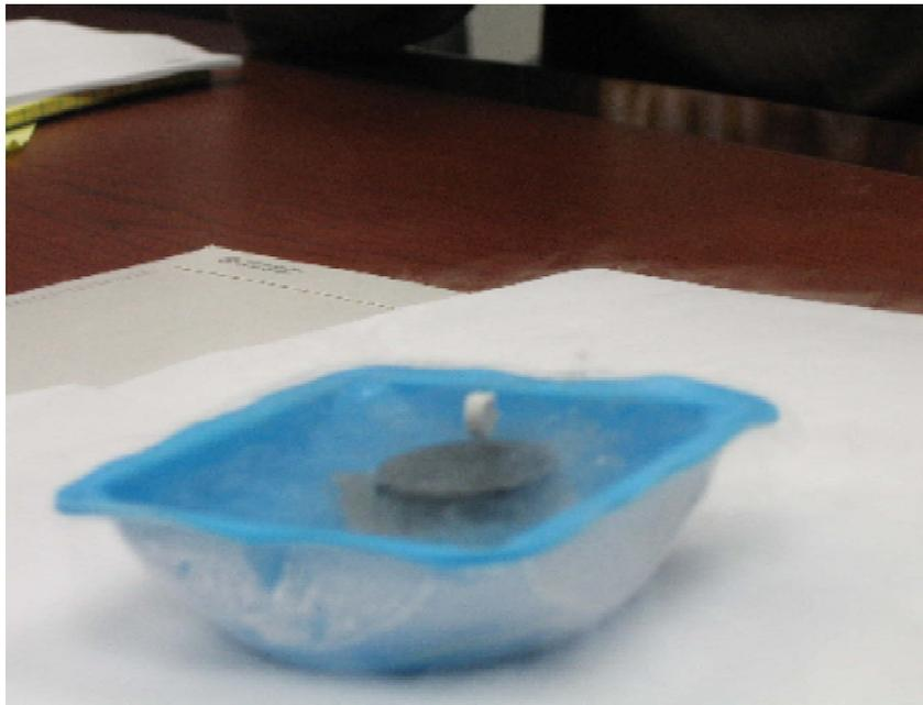
**Fig. 1(a).** Demonstration of levitation of magnet by superconducting pellet. The black disk in the blue tray of liquid nitrogen at 77 K (-320.8° F). The object floating in the mist is a small permanent magnet.
