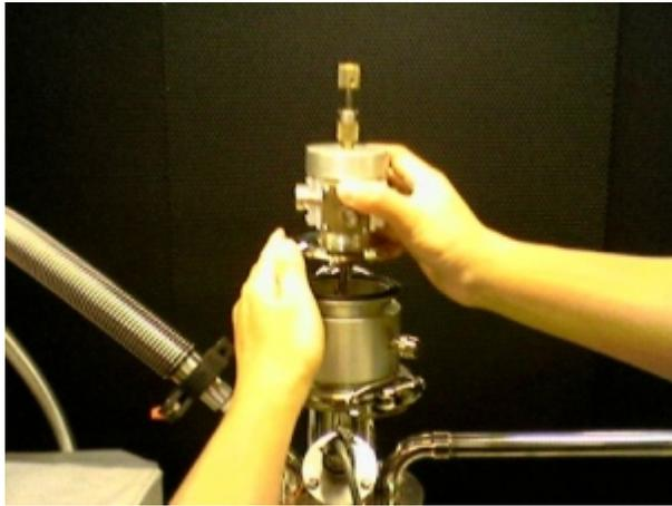
**Fig. 10.** Resistivity Measurement Apparatus showing top of cryostat with sample support rod.
