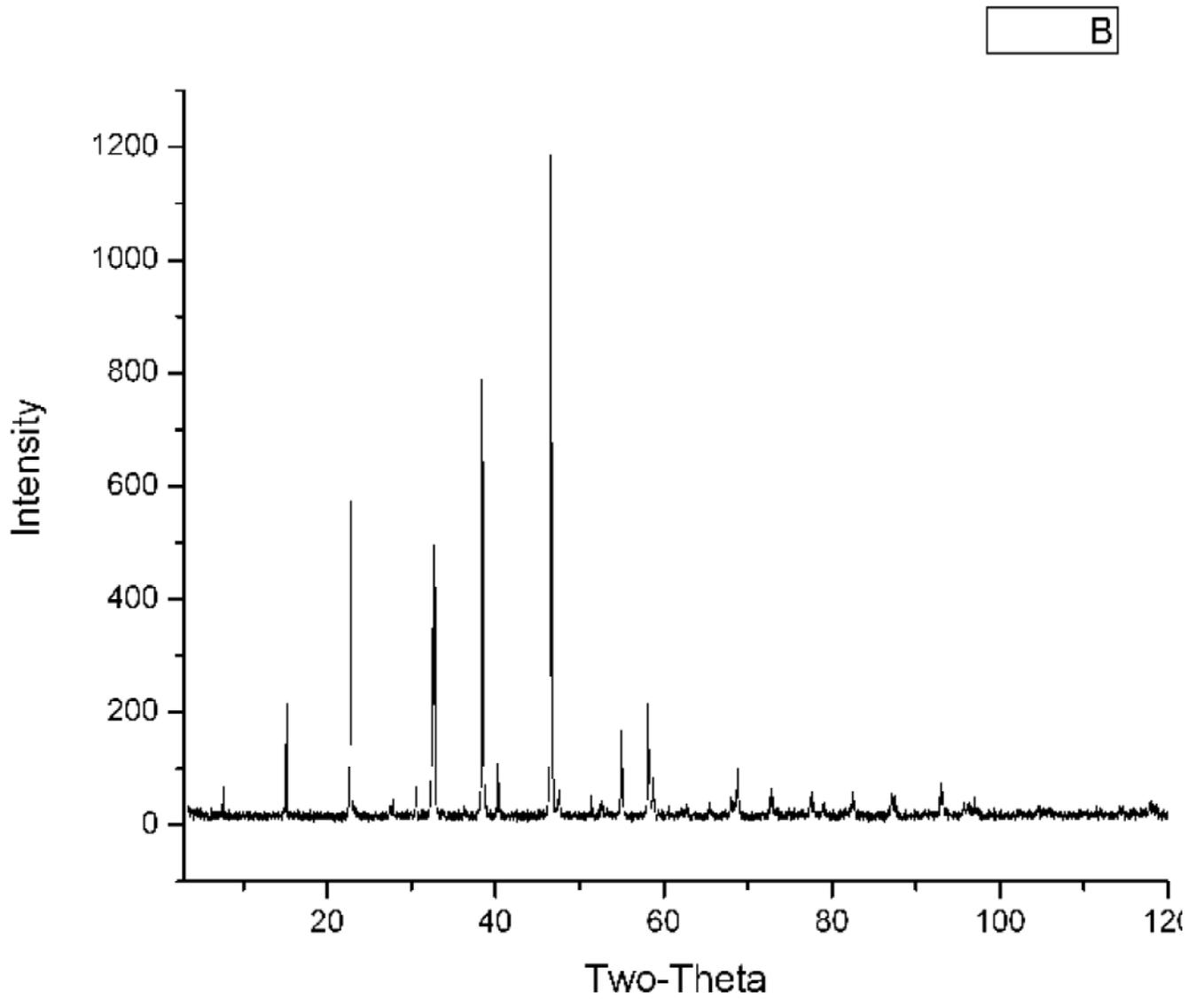
**Fig. 8.** X-Ray Diffraction pattern of the powder YBCO sample.
