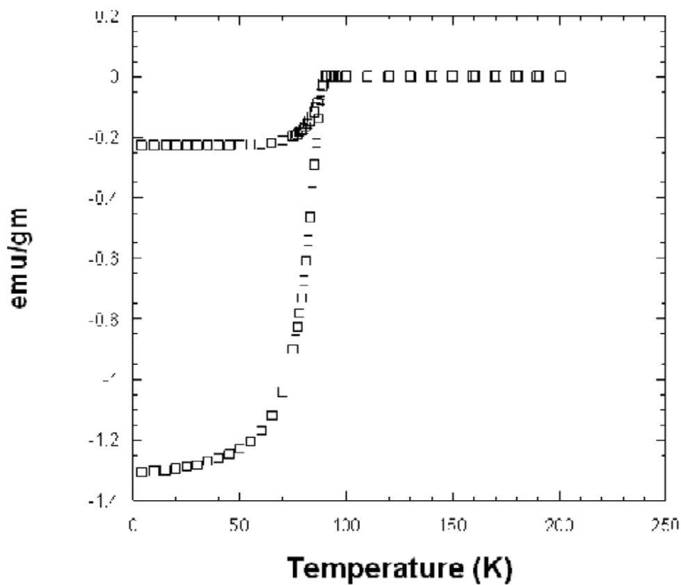
**Fig. 13.** Magnetization measurements in a 100 G field to determine the superconducting fraction of the sample. The zero field cooled portion of the plot can be used to extract the superconducting fraction. Measurements were conducted at Prof. M. Greenblatt's Lab. at Rutgers University.
