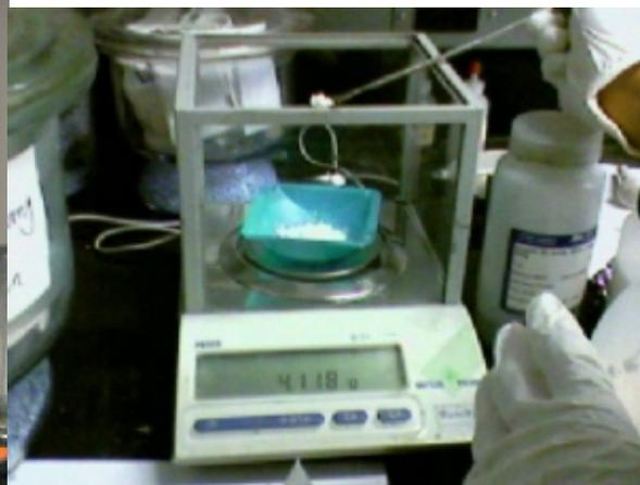
**Fig. 3.** Weighing the components ( $Y_2O_3$ ,  $CuO$  and  $BaCO_3$ ), needed to get the correct stoichiometric ratio for YBCO ( $YBa_2Cu_3O_{6+x}$ ).
