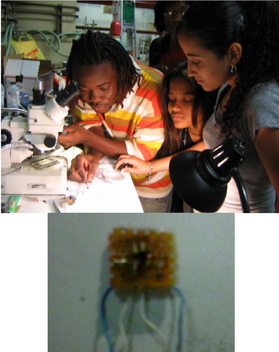
**Fig. 9.** Preparing a rectangular (polished) sample for Resistivity measurements. Rectangular sample as placed on circuit board.
