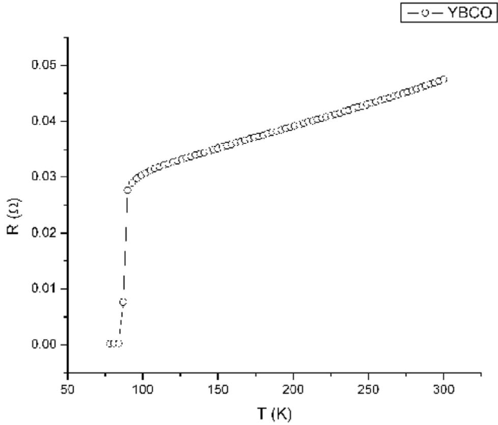
**Fig. 11.** Resistance as a function of temperature for the sample can be converted to resistivity using the measured sample dimensions.
