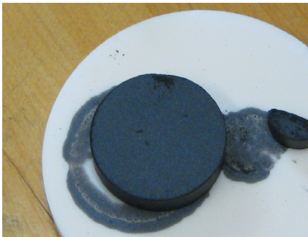
Fig. 4. Two pellets were produced: one for testing for the Meissner effect (large one) and one used in parts for resistivity, Raman and magnetization measurements.
