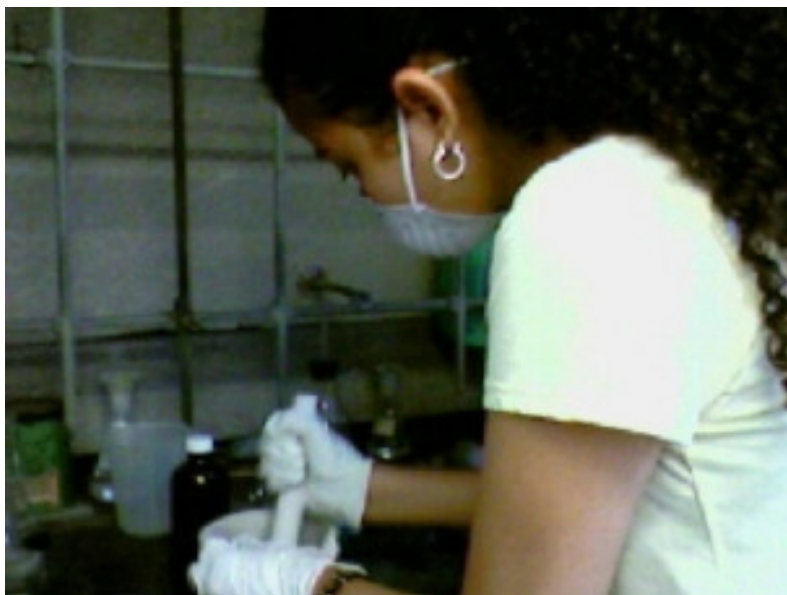
Fig. 3. Monica (from 2007) grinding powder for first calcinations sample as a example of the procedure. After grinding for 45 minutes to produce a uniform grey powder the sample was heated in air for ~24 hours at 950^{\circ} C. This was repeated 3 times and the sample was then pressed into a pellet for the final heating.
