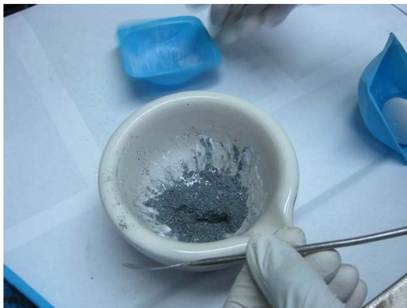
Fig. 2. Students weighed the starting materials ( \text{CuO} , \text{Y}_2\text{O}_3 and \text{BaCO}_3 ) of appropriate ratios for synthesis of YBCO (top) and mixed them (bottom) with a spatula before grinding the powder for 45 minutes in the mortar and pestle. The sample was heated to 850^\circ\text{C} for \sim 12 hrs. ground again for 45 minutes three consecutive times and then pressed into a small and large pellet for extensive testing. Approximately 1 week is required to prepare a sample.
