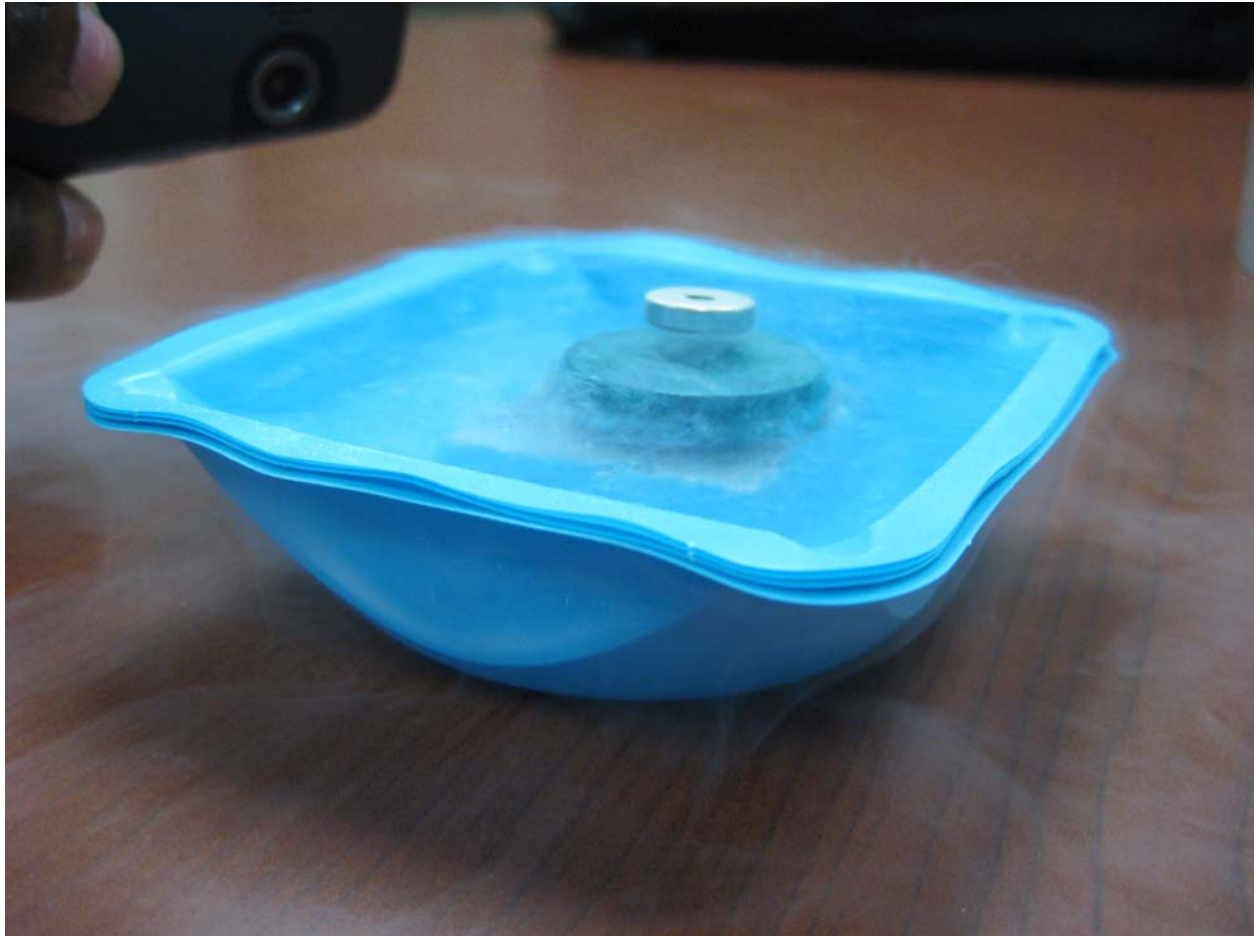
Fig. 7. Meissner Effect test on sample (black pellet covered by liquid nitrogen) to definitively show that the sample superconducts and expels the field of the magnet causing it to float above the YBCO pellet.
